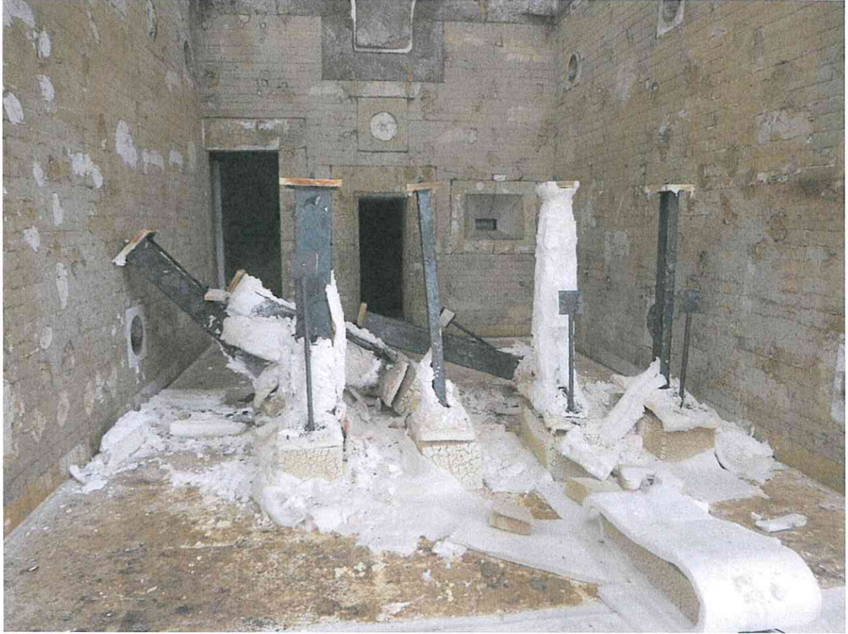
Photo C2: The aspect of columns after the test
