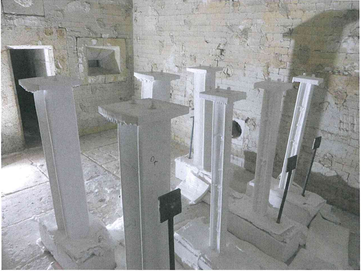
Photo C1: The aspect of columns before the test
