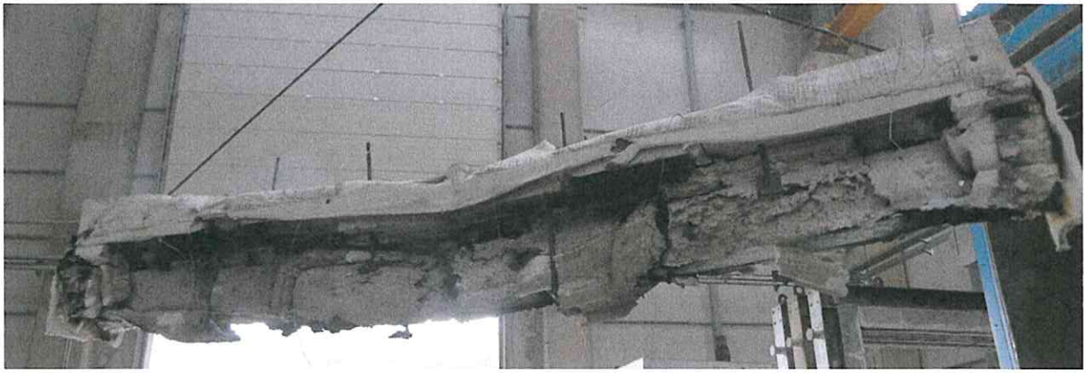
Photo C2: The aspect of the loaded beam after the test
